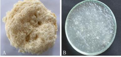
A: High water absorbing cassava starch phosphate carbamate; B: Microgel after water absorption
